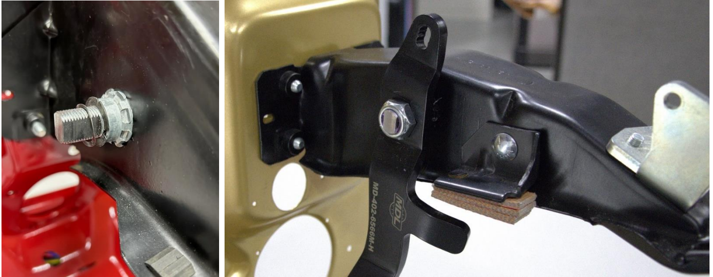
MDL supplied clutch pedal shown installed. Cylinder and brake pedal not shown for clarity.
