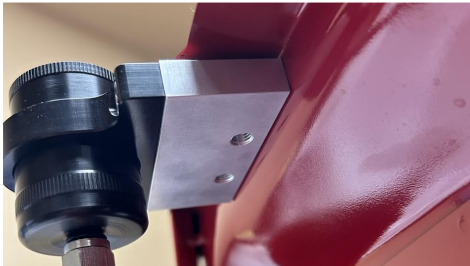
Black billet reservoir shown with optional clear billet spacer, mounted through the firewall.
